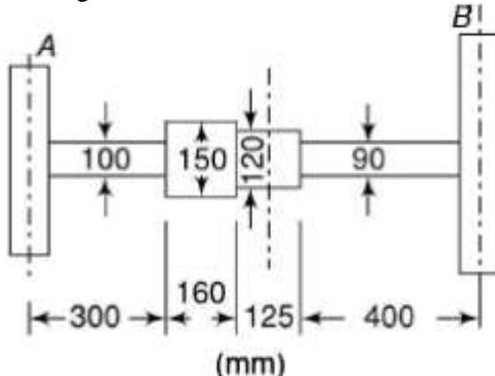
The mass A is 300 kg with a radius of gyration of 0.75 m and the mass B is 500 Kg with a radius of gyration of 0.9 m. Determine the frequency of the torsional vibrations. It is desired to have the node at the mid-section of the shaft of 120 mm diameter by changing the diameter of the section having a 90 mm diameter. What will be the new diameter?
