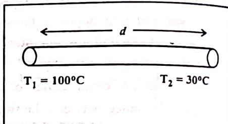
$$Q = \frac{kA(T_1 - T_2)t}{d}$$
