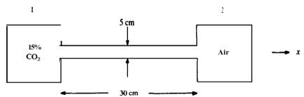
Both tanks are at 1 atmospheric pressure and 298.15 K. The volume of each tank is large compared to the volume of gas in the 30 cm connection line so concentration changes in each tank are negligible for a very long time after the beginning of the experiment. The diffusion coefficient of CO<sub>2</sub> in air at 1 atm. and 25°C is 0.164×10<sup>4</sup> m<sup>2</sup> s<sup>-1</sup>. Calculate the initial rate of mass transfer of the CO<sub>2</sub>?
